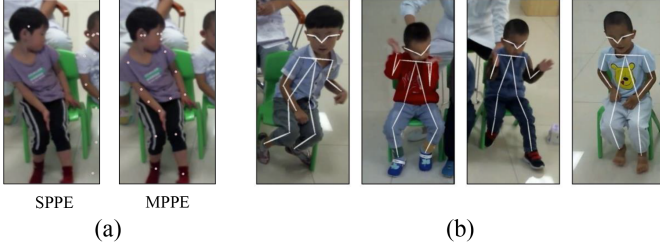
Fig. 4. (a) Visualization of Pose Estimation Methods. SPPE means single-person pose estimation method, and MPPE means multi-person pose estimation. (b) Visualization of pose estimation by AlphaPose.
